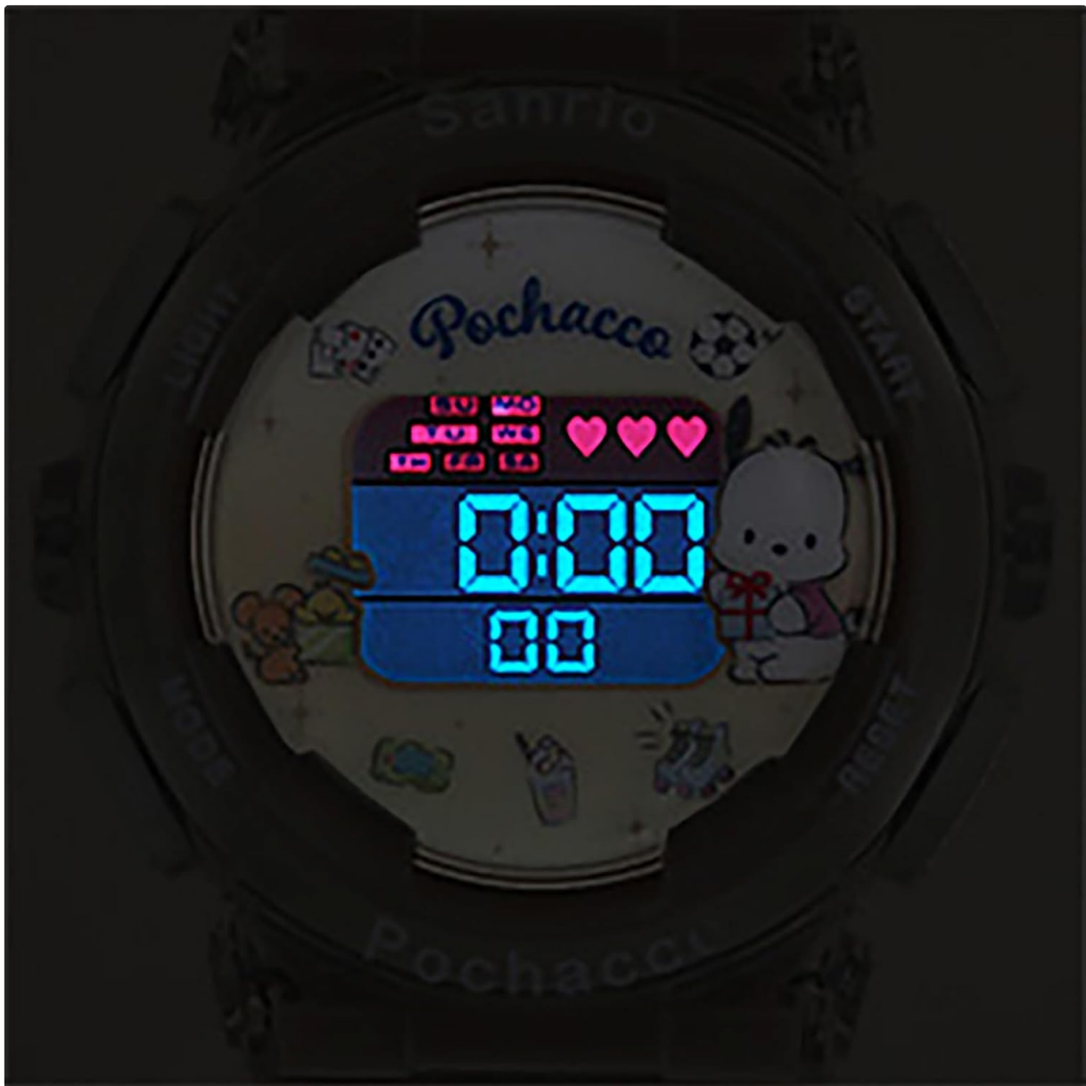
Image 3.1: The watch display with the EL backlight active, providing clear visibility in the dark.
