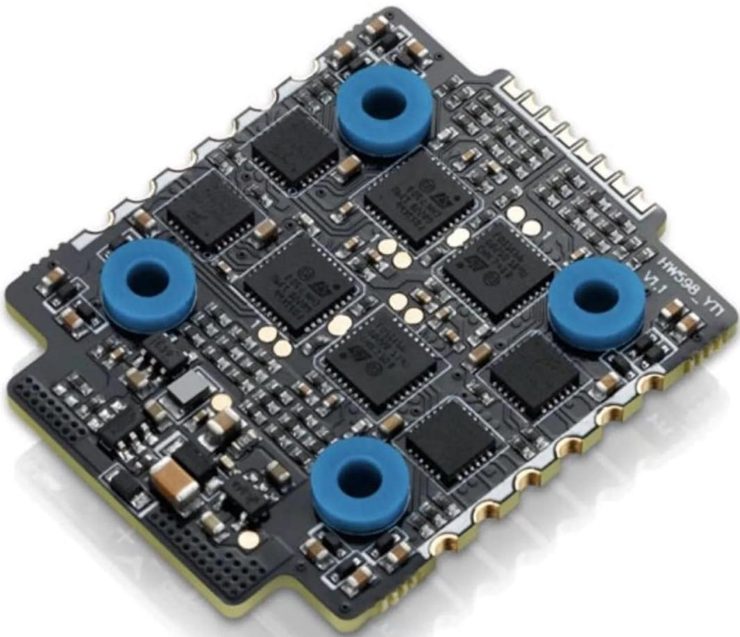
**Figure 1:** Top view of the HOBBYWING XRotor FPV 45A G2 ESC (4in1). This image displays the main components, including the microprocessors and capacitors, along with the four blue damping rings for mounting.
