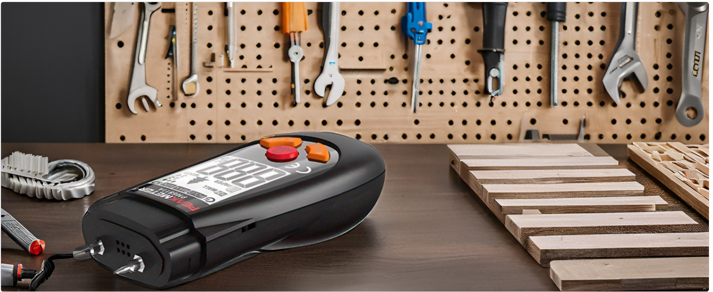
Figure 5.2: The display changes color to indicate moisture levels: green for low, yellow for medium, and red for high.
