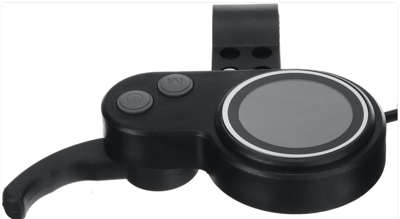
Figure 2: Close-up view of the control panel, highlighting the power button (top right) and mode button (bottom right) next to the
