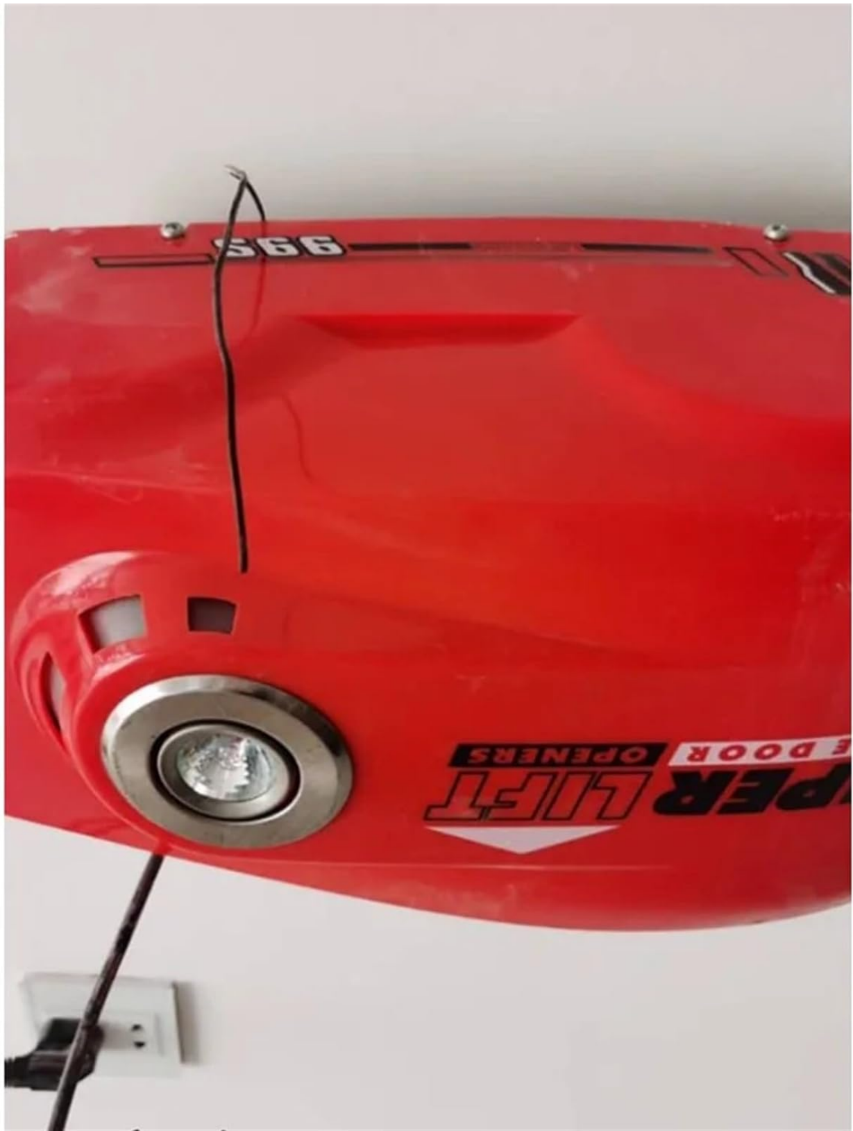
Figure 4.1: An example of a Spreit SUPERLIFT S66 garage door opener unit, which this transformer is designed to power. This image shows the red casing of the opener mounted to a ceiling, with a light fixture and wiring visible.
