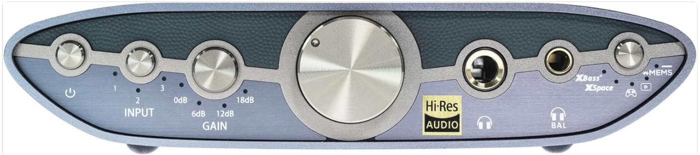
Figure 4.1: Front Panel Layout of the iFi Zen CAN 3
