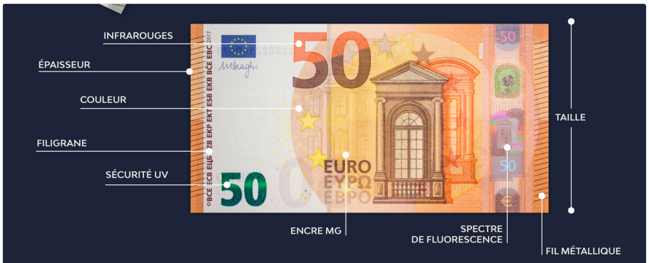
Image: Visual representation of the advanced detection technologies, including infrared, UV security features, magnetic ink, and other physical characteristics used to verify banknote authenticity.
