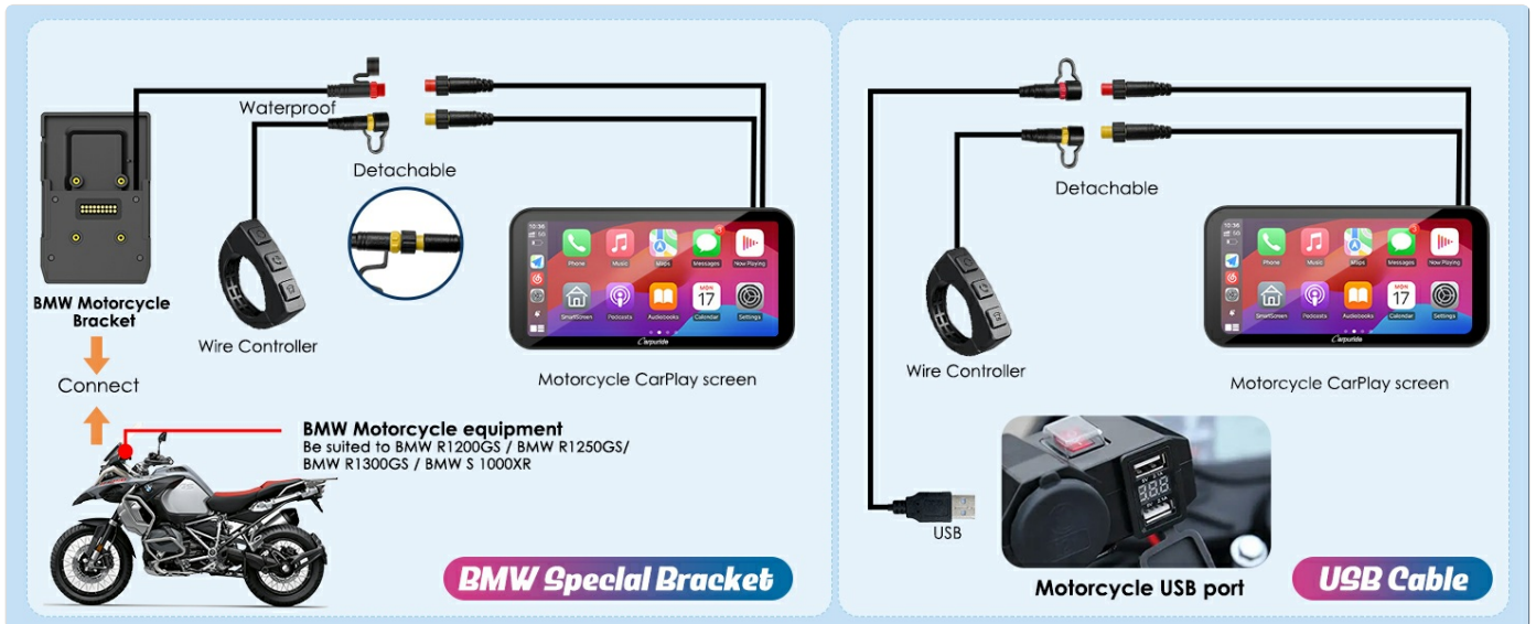
Figure 4: Power connection options for the Carpuride W603B.
