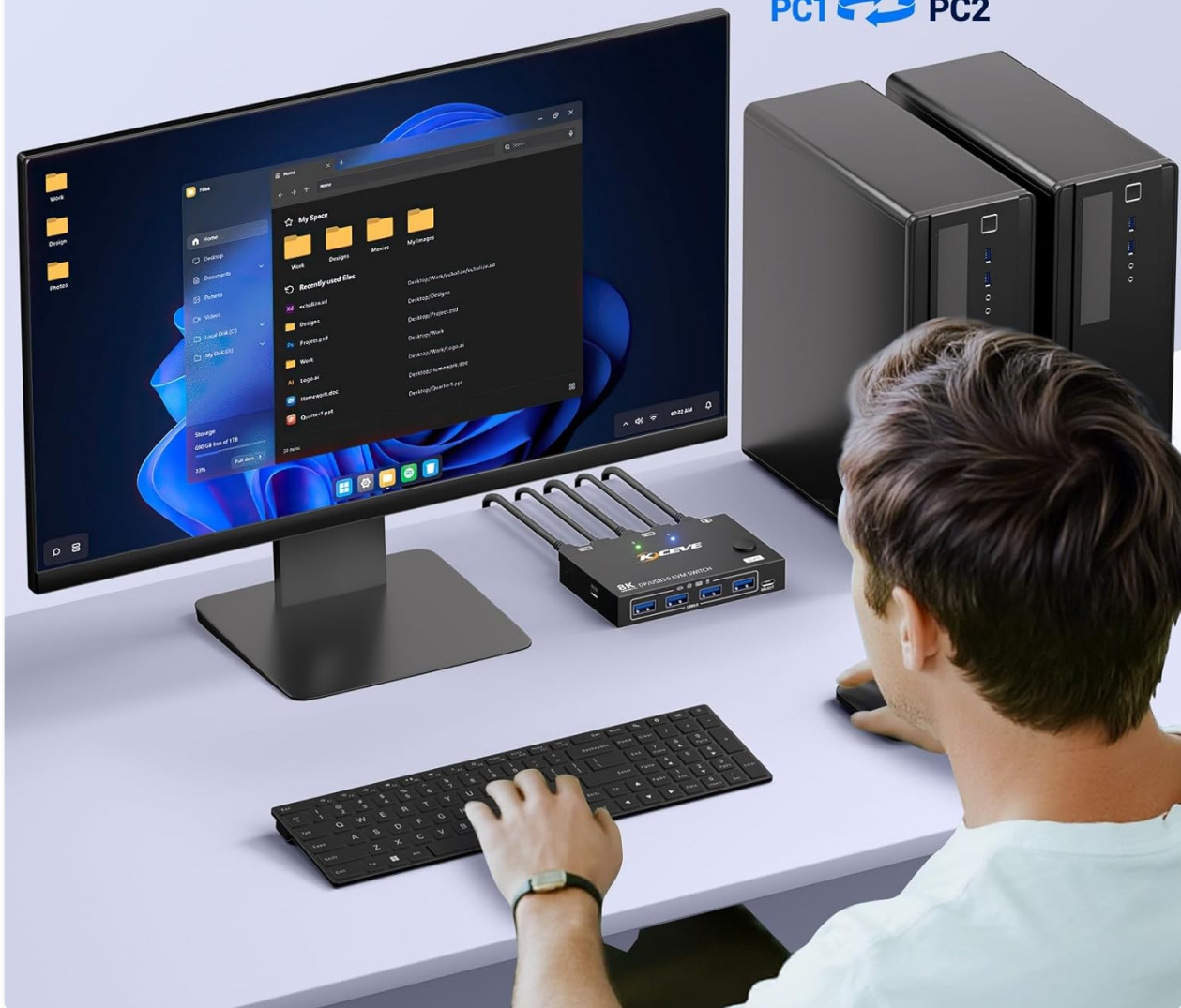
Figure 4: Example setup showing two computers sharing a single monitor and peripherals via the KVM switch. This image demonstrates a typical setup, showing two desktop computers connected to the KVM switch, which then connects to a single monitor, keyboard, and mouse, enabling shared access.
