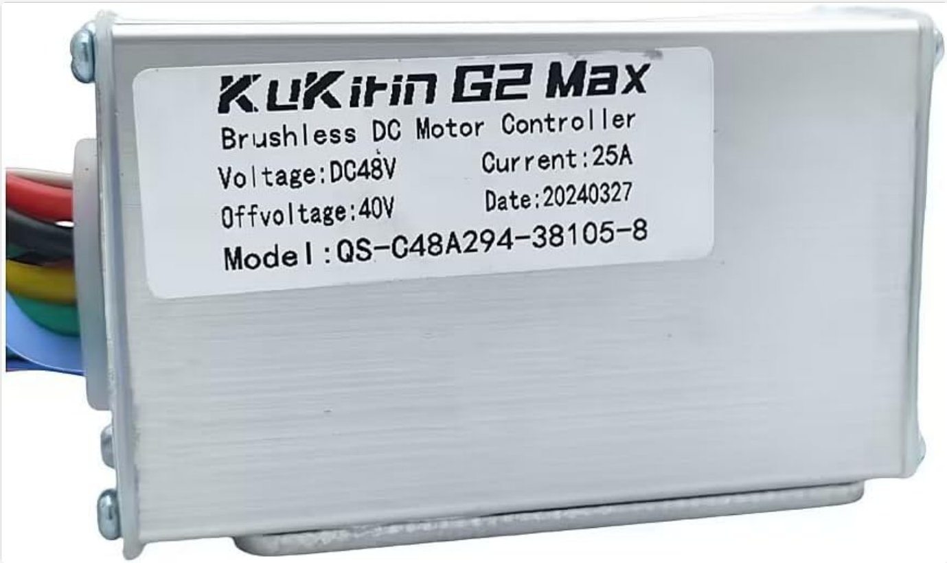
Image 8.1: A close-up of the controller's label, displaying critical operational parameters.
