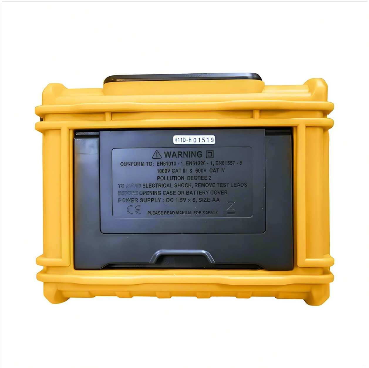
Figure 2.1: Rear view of the MS5910, highlighting the battery compartment and safety warning label.
