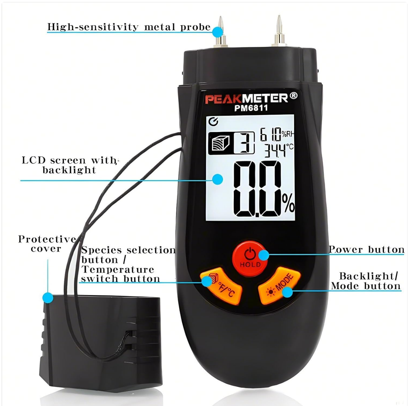
Figure 1: PEAKMETER PM6811 with labeled components. This image shows the high-sensitivity metal probes, LCD screen with backlight, protective cover, power button, species selection button/temperature switch button, and backlight/mode button.
