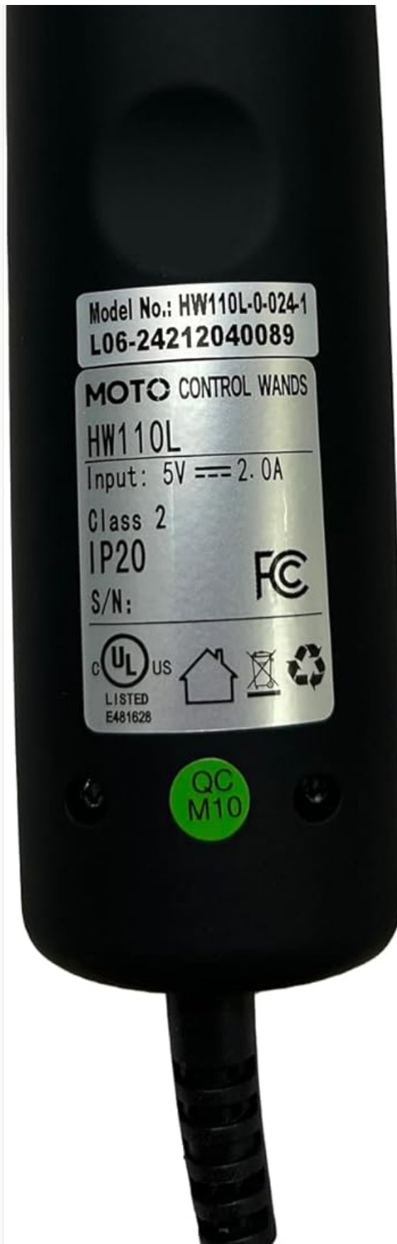
Image 7.1: The back of the remote control, displaying manufacturing details, model number (HW110L), and electrical input specifications.
