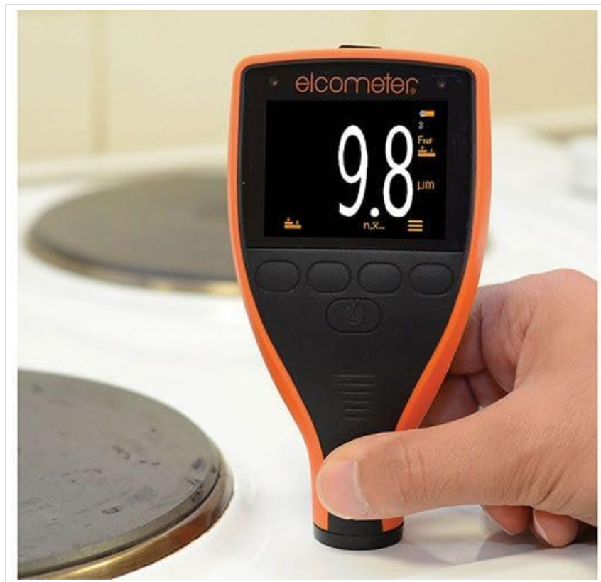
Figure 2: The Elcometer 415 Gauge being used to measure the thickness of a coating on a flat surface.
