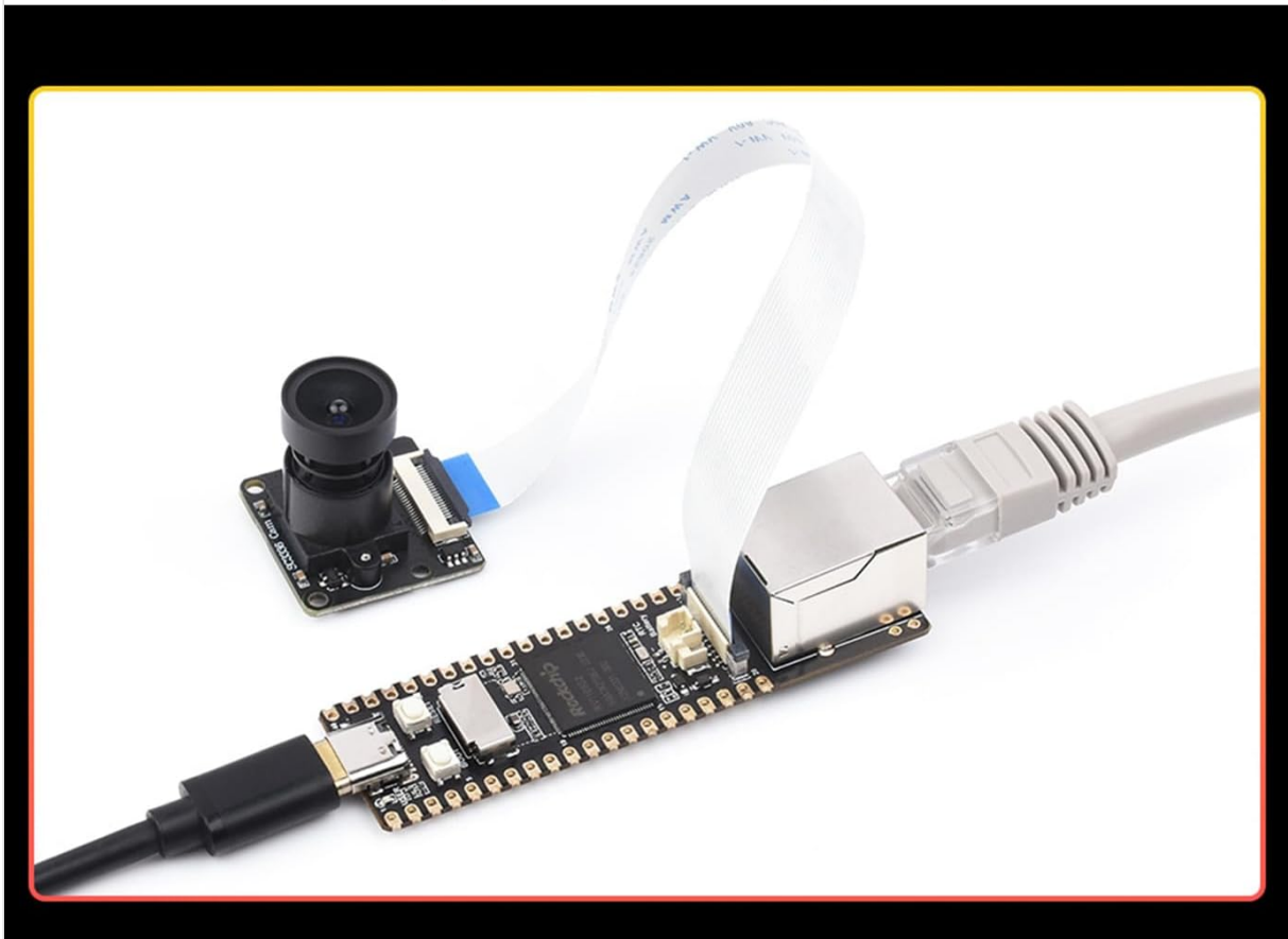
Figure 7: An example application setup showing the Luckfox Pico Pro connected to a camera module via MIPI CSI and to an Ethernet cable, demonstrating its capability for vision and network-enabled projects.
