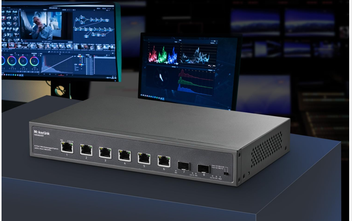
Image 1.1: Front view of the MokerLink 8-Port 10Gbps Ethernet Switch, highlighting its 6x 10Gbps RJ45 ports and 2x 10Gbps SFP+ ports.
