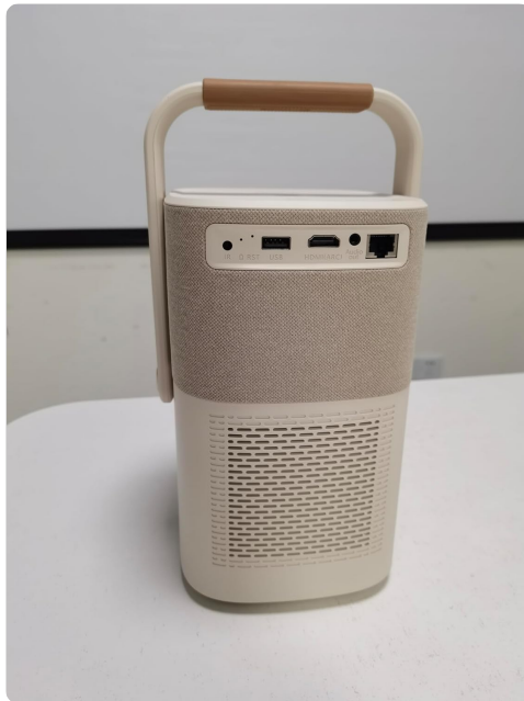
Figure 2.2: Rear View. Displays the various input/output ports including IR receiver, Reset button, USB, HDMI (ARC), Audio Out, and Ethernet.
