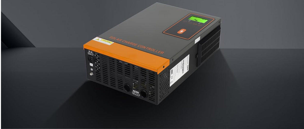
Figure 1.2: Overview of the 140A MPPT Charge Controller's key features, highlighting its 48V system support, 6500W max PV array power, 500V max PV VOC, compatibility with Lead-acid and Lithium batteries, and configurable charging current.
