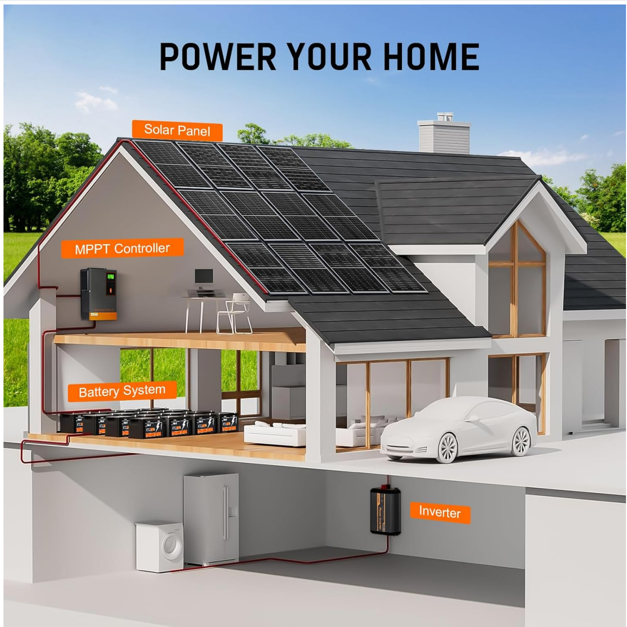
Figure 7.2: Illustrative diagram showing how the Temank MPPT Controller integrates into a home solar power system, connecting solar panels to a battery system and an inverter to power household appliances.
