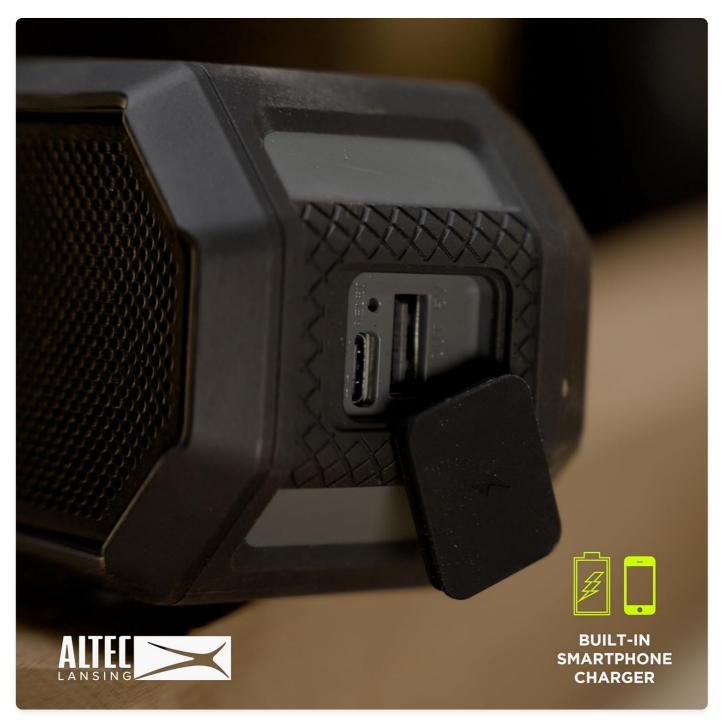
The USB-C input and USB-A output ports for charging and power bank functionality.
