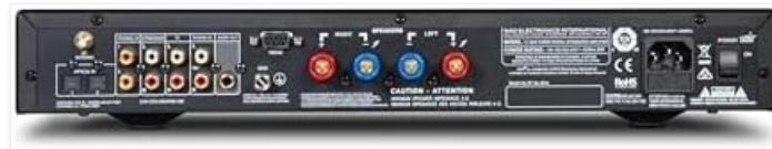
Image 3.2: Rear panel of the NAD C 328 Integrated Amplifier, illustrating speaker terminals, analog and digital inputs, and power connection.
