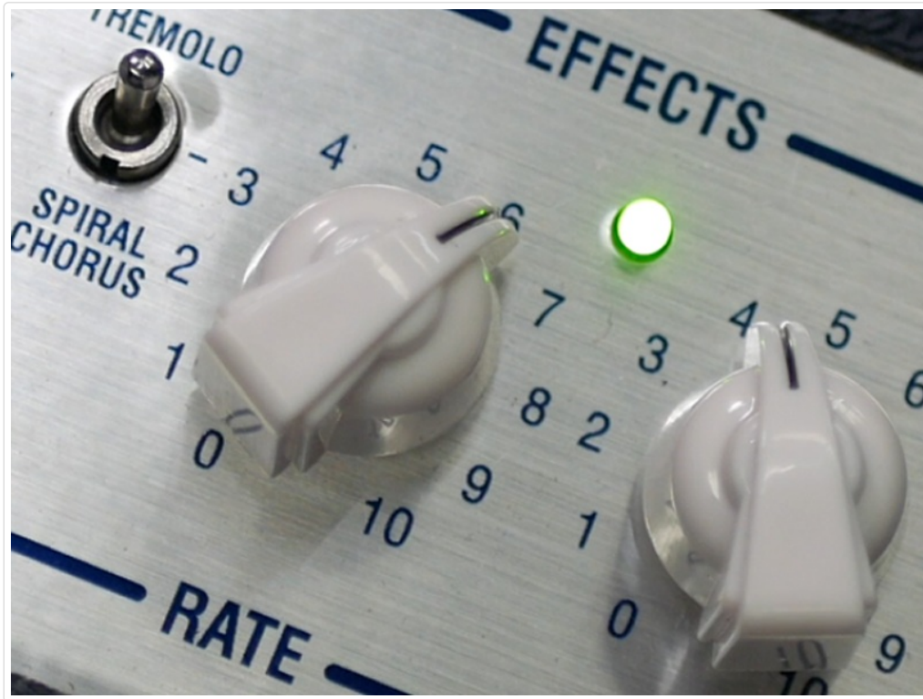
Figure 6: Detail of Reverb, Tremolo/Chorus switch, Rate, and Depth controls.
