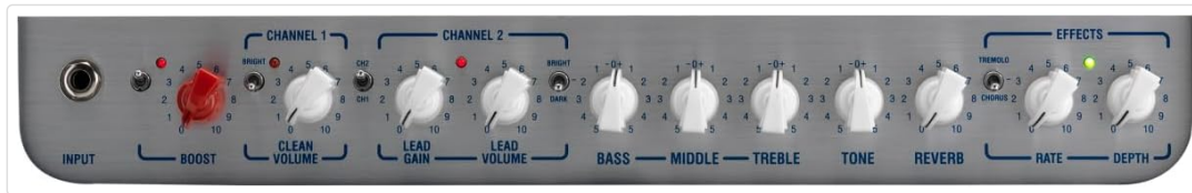
Figure 1: Overview of the amplifier's front control panel.
