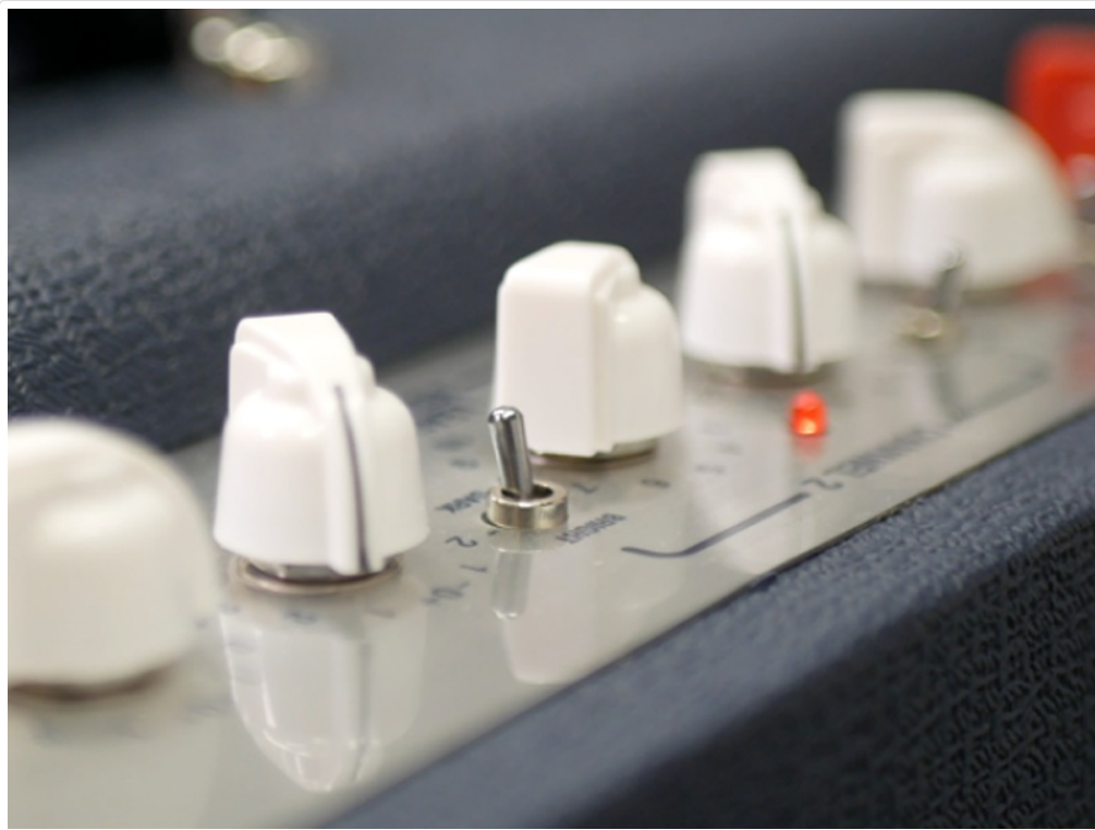
Figure 3: Detail of Channel 1 controls including Boost, Clean Volume, and Bright switch.
