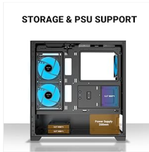
Figure 4: Locations for 3.5" HDDs, 2.5" SSD, and Power Supply Unit (PSU) with 200mm clearance.
