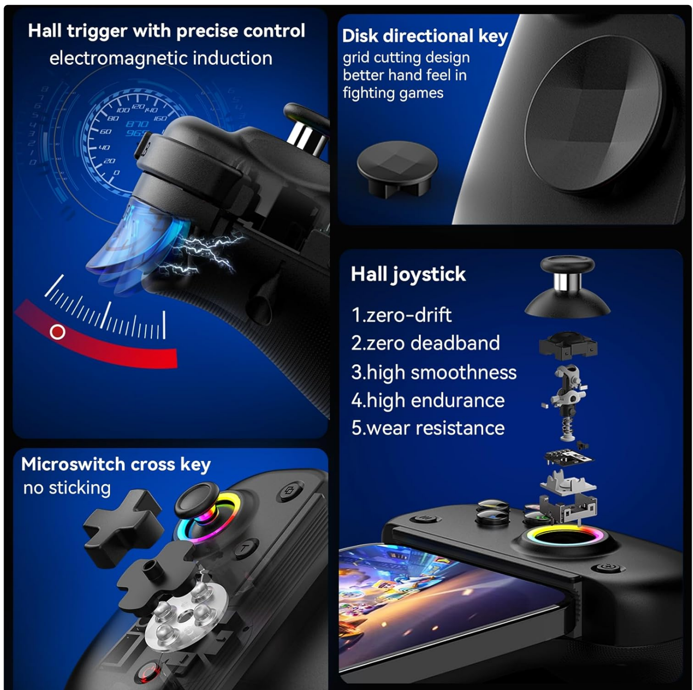
Image: Exploded view highlighting the Hall trigger, Hall joystick, disk directional key, and microswitch cross key for precise control.
