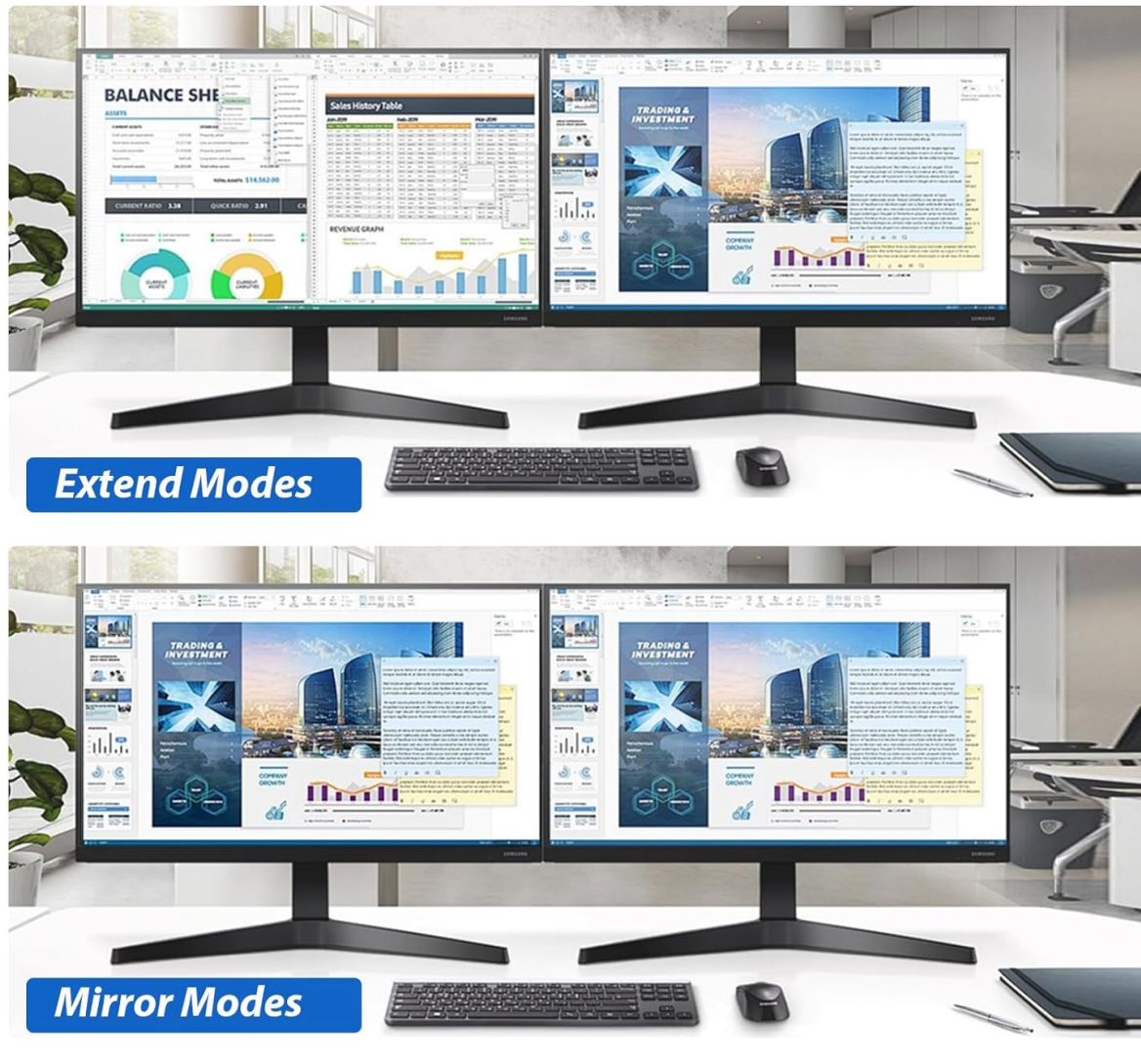
Figure 5: This image illustrates the Extended and Mirror display modes supported by the KVM switch. Extended mode shows different content on each monitor, while Mirror mode duplicates content across both.
