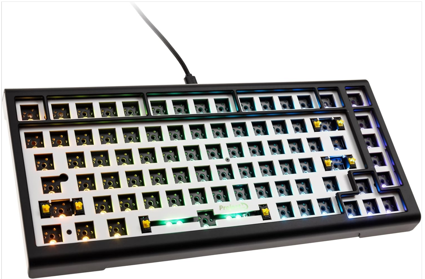
Image: Top view of the Ducky ProjectD Tinker 75 RGB Barebone Mechanical Keyboard, showcasing its 75% layout and empty switch sockets.
