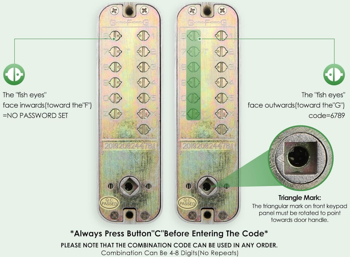
Image 5.2: Code Setting Mechanism
