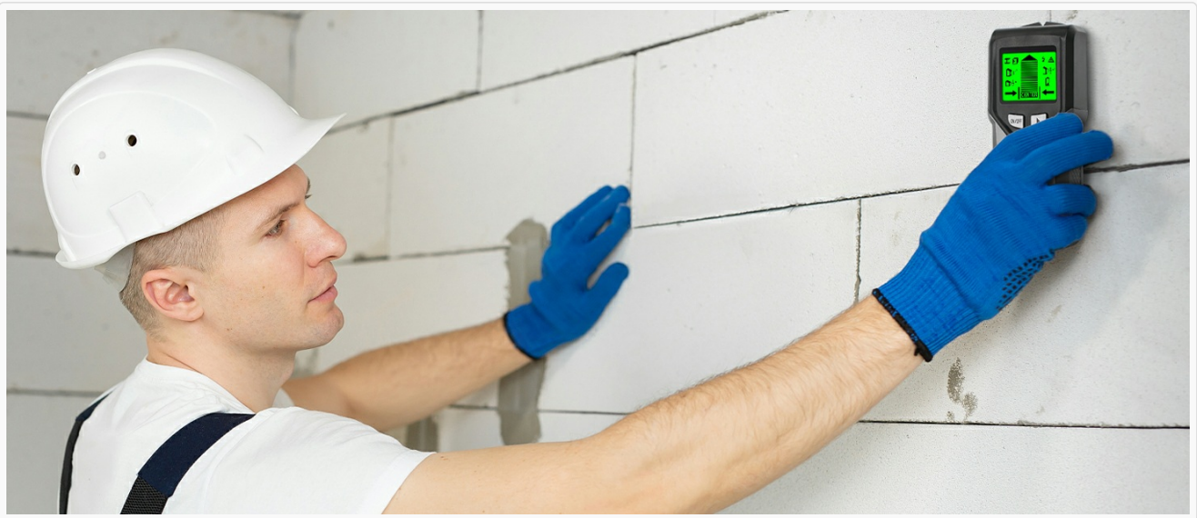
Image 7: Visual guide demonstrating the process of using the AC scan mode to detect live electrical wires within a wall.
