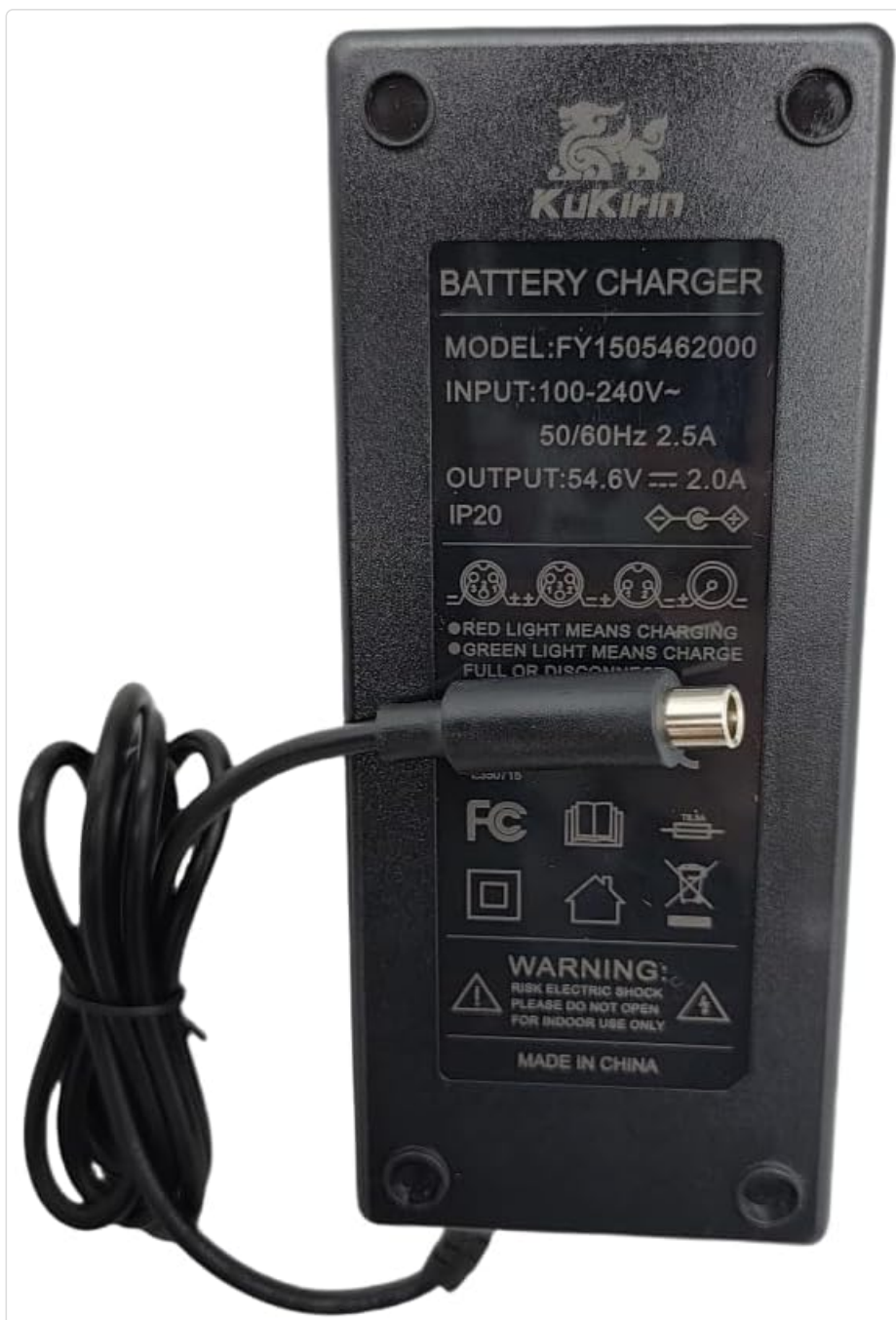
Image 8.1: Close-up of the charger's label, confirming model number, electrical ratings, and compliance marks.
