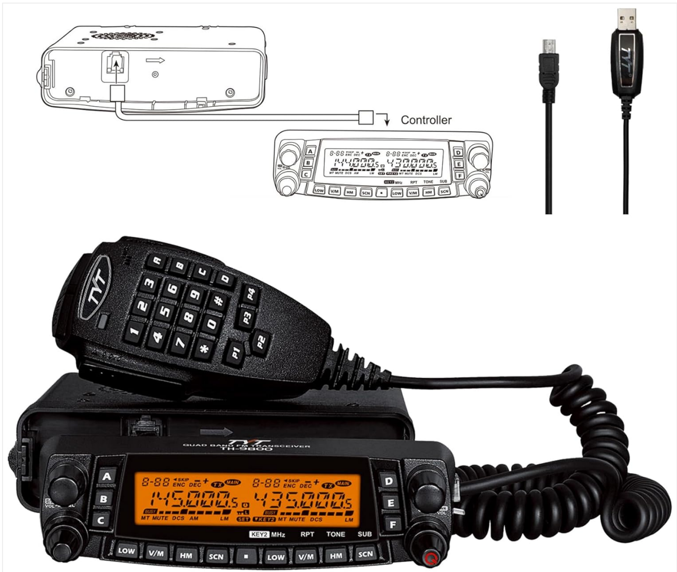
Image 4.1: Detachable Front Panel Connection. This diagram illustrates how the front control panel connects to the main radio unit via the separation cable, allowing for flexible mounting options.
