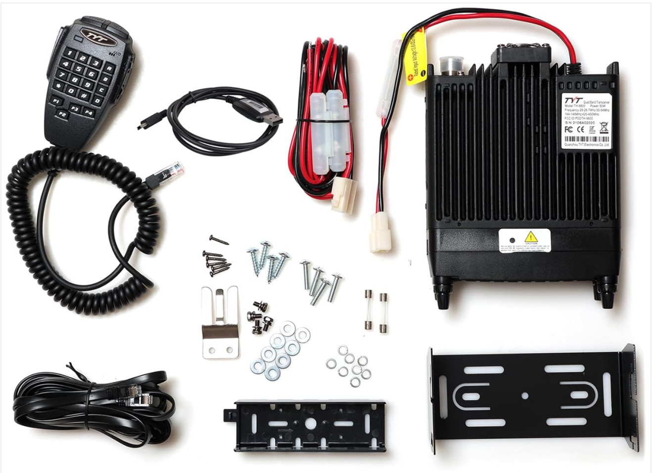
Image 2.1: Package Contents. This image displays all components included with the VMUKSAN TYT TH-9800 Plus mobile radio, laid out for easy identification. These include the main transceiver unit, microphone, various cables, mounting brackets, screws, and fuses.
