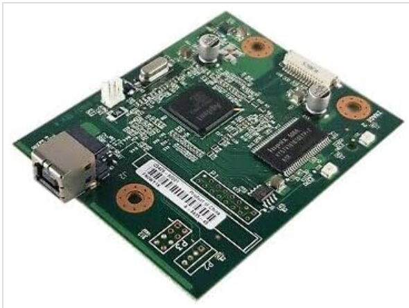
Figure 2.1: Top view of the Generic Replacement HP LaserJet Formatter Board (CB409-60001-RO). This image shows the green circuit board with various electronic components, including chips, capacitors, and connectors, such as a USB port and internal ribbon cable connectors. A barcode label is visible on the board.
