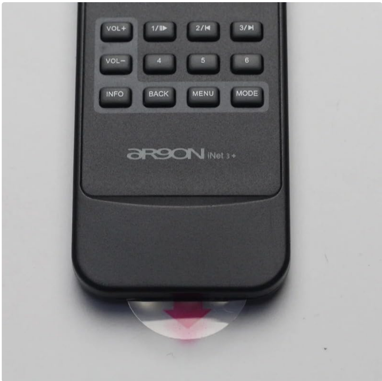
Figure 2: Clear plastic tab (battery insulator) to be removed from the bottom of the remote.
