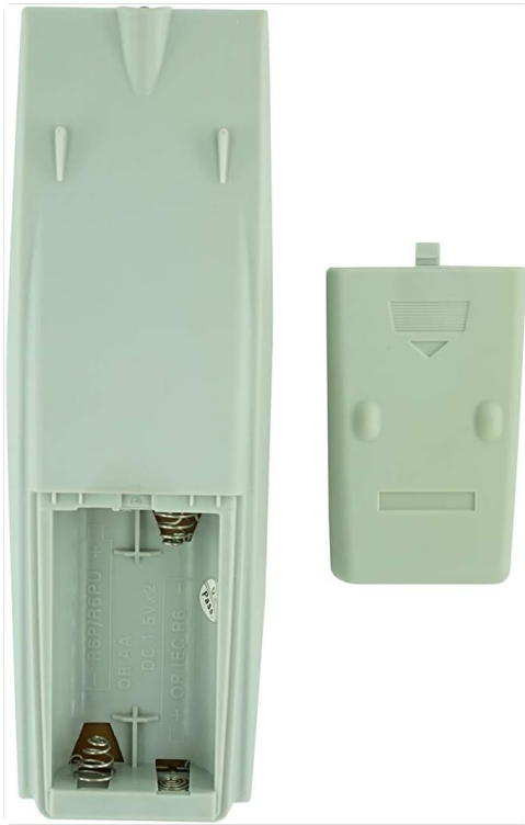
Figure 2: Battery compartment with cover removed, ready for battery insertion.
