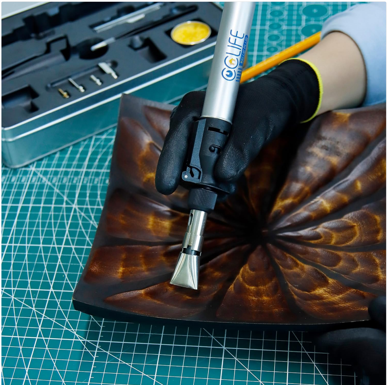
Image 6.3: The heat blower attachment is demonstrated, applying heat to a surface, suitable for tasks like heat shrinking.
