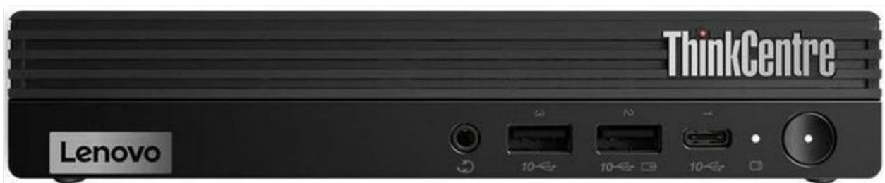
Figure 1: Front view of the ThinkCentre M75q Gen 5, highlighting the power button, USB ports, and audio jack.
