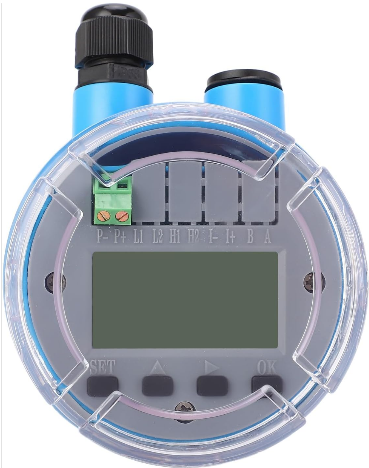
Image 6.1: Top-down view of the sensor's control panel, showing the terminal block and LED display. This image clearly labels the power input (P-, P+) and analog output (I-, I+) terminals, along with the touch keys (SET, UP, DOWN, OK) for parameter configuration.
