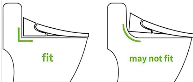
Figure 2: Toilet Fit Check Guide. Ensure your toilet matches the "Round" dimensions for optimal fit.
