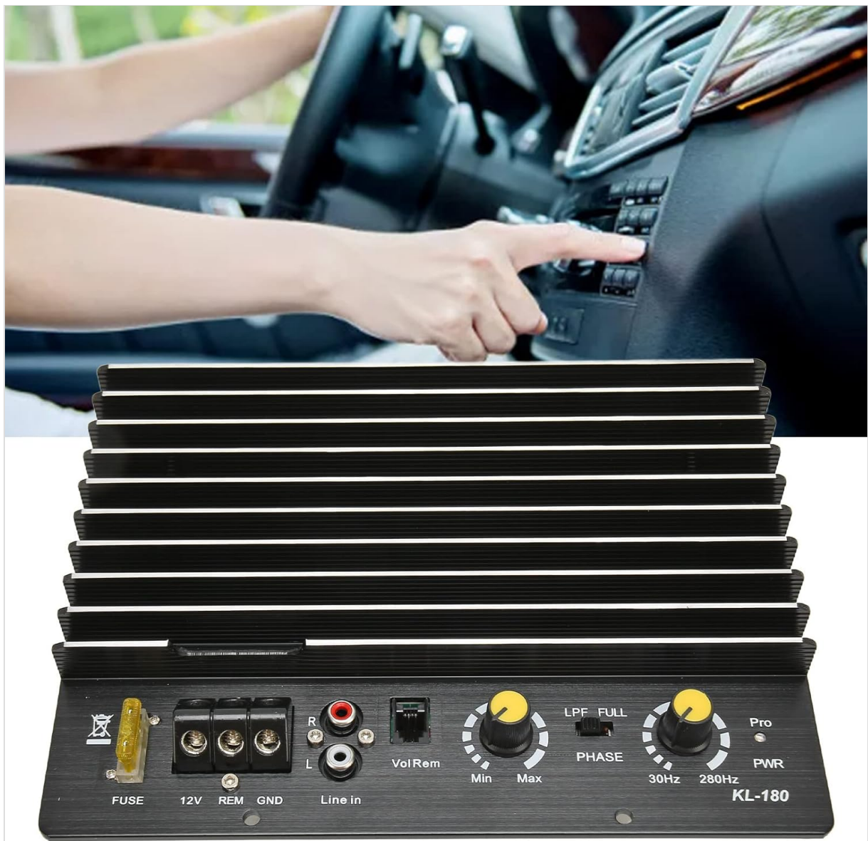
Figure 4.1: Front view of the Diyeeni Car Amplifier Board KL 180, showing the control panel with FUSE, 12V, REM, GND terminals, Line In (RCA), Vol Rem, LPF/FULL/PHASE switch, 30Hz-280Hz frequency knob, and PWR indicator. The heat sink fins are prominent.
