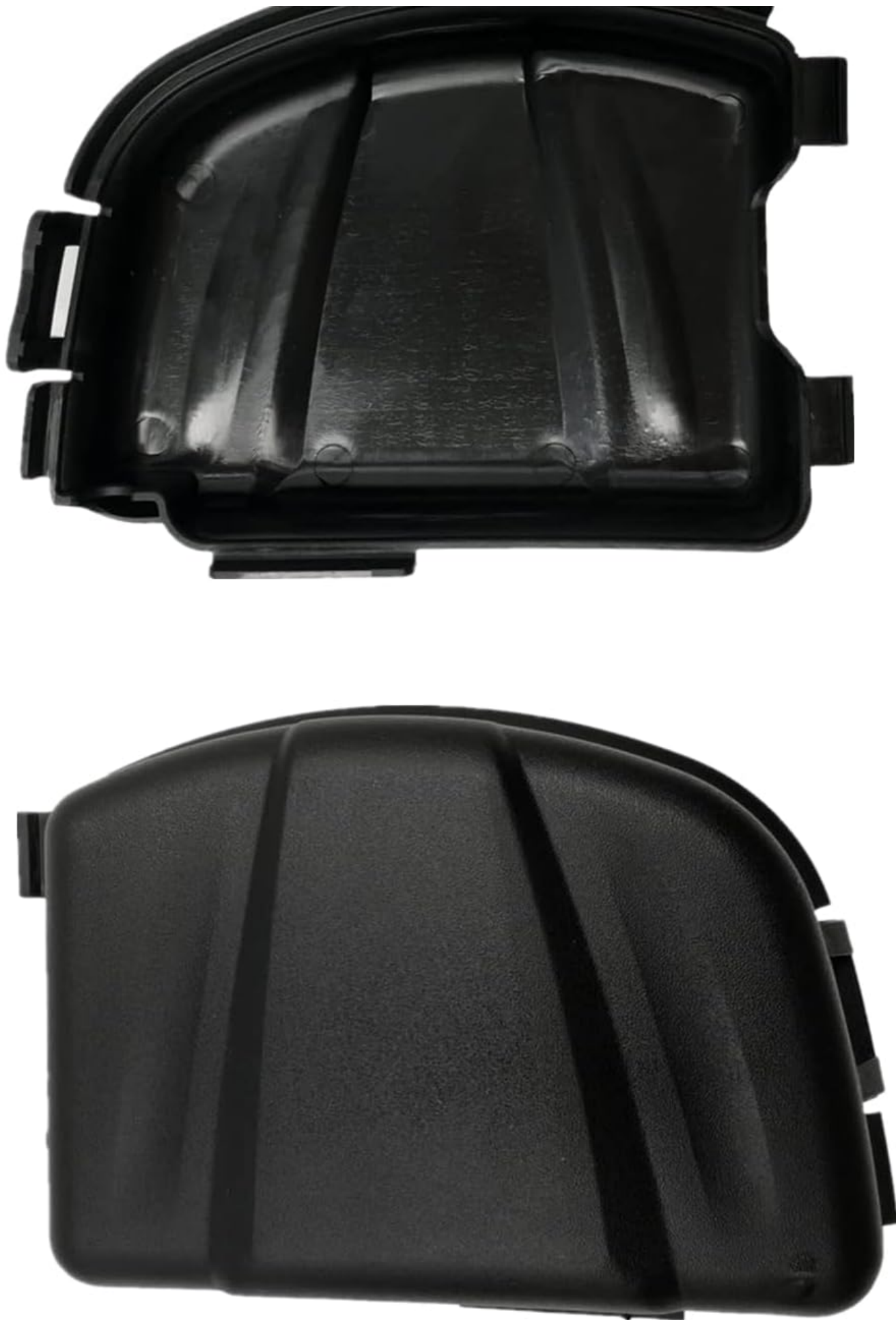
Figure 3.2: The air filter cover, which protects the air filter element.
