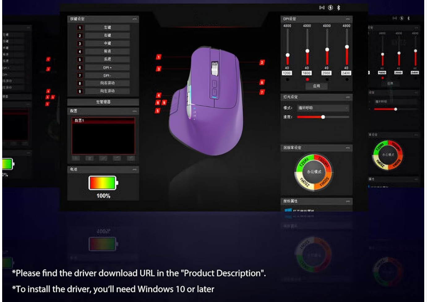
Image 5.4: Driver Software Interface. This image displays the user interface of the driver software for the TISHLED TM015-P mouse. It shows options to set DPI, lighting effects, report rate, and macros, allowing for comprehensive customization of the mouse's 9 programmable buttons.
