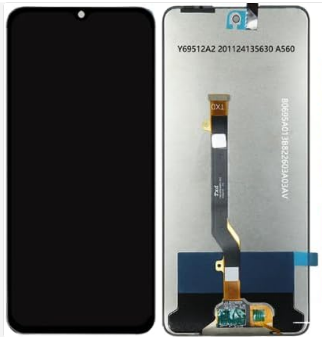
Figure 2.2: Rear view of the replacement screen, highlighting the flex cable connection points.
