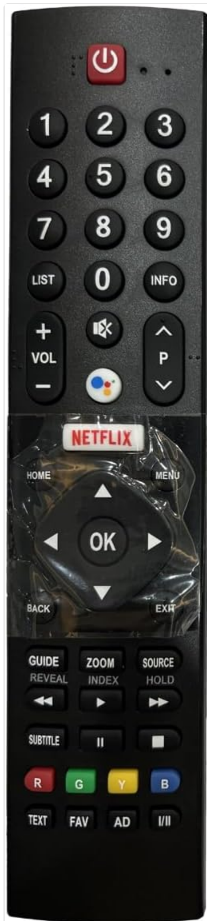
Figure 1: Overview of the GHUST Voice Remote Control. This image displays the full remote, showing the power button, number pad, volume and channel controls, navigation buttons, and dedicated function keys.
