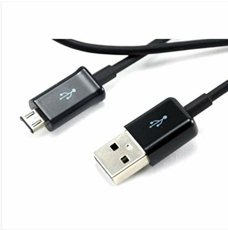
Figure 2: Detailed view of the MicroUSB and USB-A connectors, highlighting their distinct shapes.
