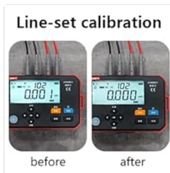
Figure 5.4.1: Line-Set Calibration. Illustrates the difference in readings before and after performing a line-set calibration.
