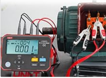
Figure 5.2.3: Four-Wire Measurement Method. Visual representation of how the four leads are connected for accurate resistance measurement.
