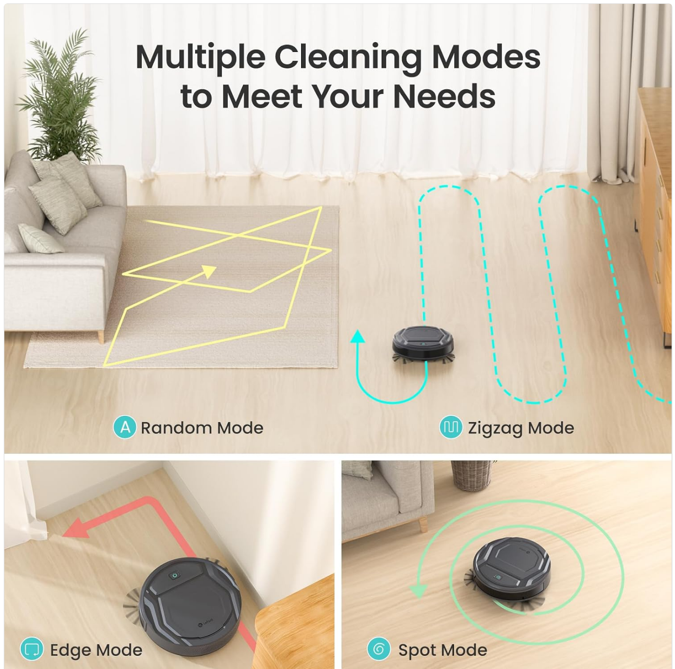
Image: Illustrations of the robot vacuum performing different cleaning patterns: Random Mode, Zigzag Mode, Edge Mode, and Spot Mode.
