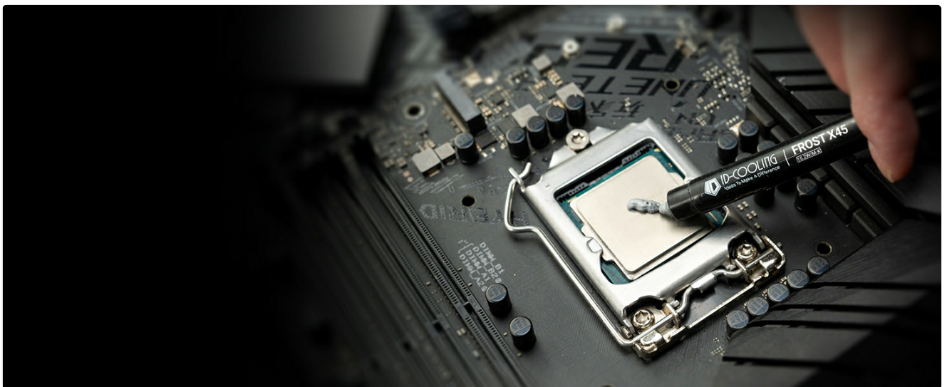
Figure 3.2: Application of thermal paste on the CPU surface.
