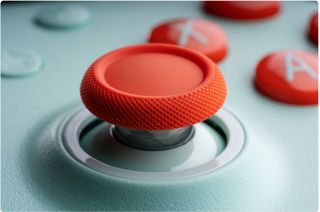
Figure 5: Hall Effect Joysticks for improved precision.
