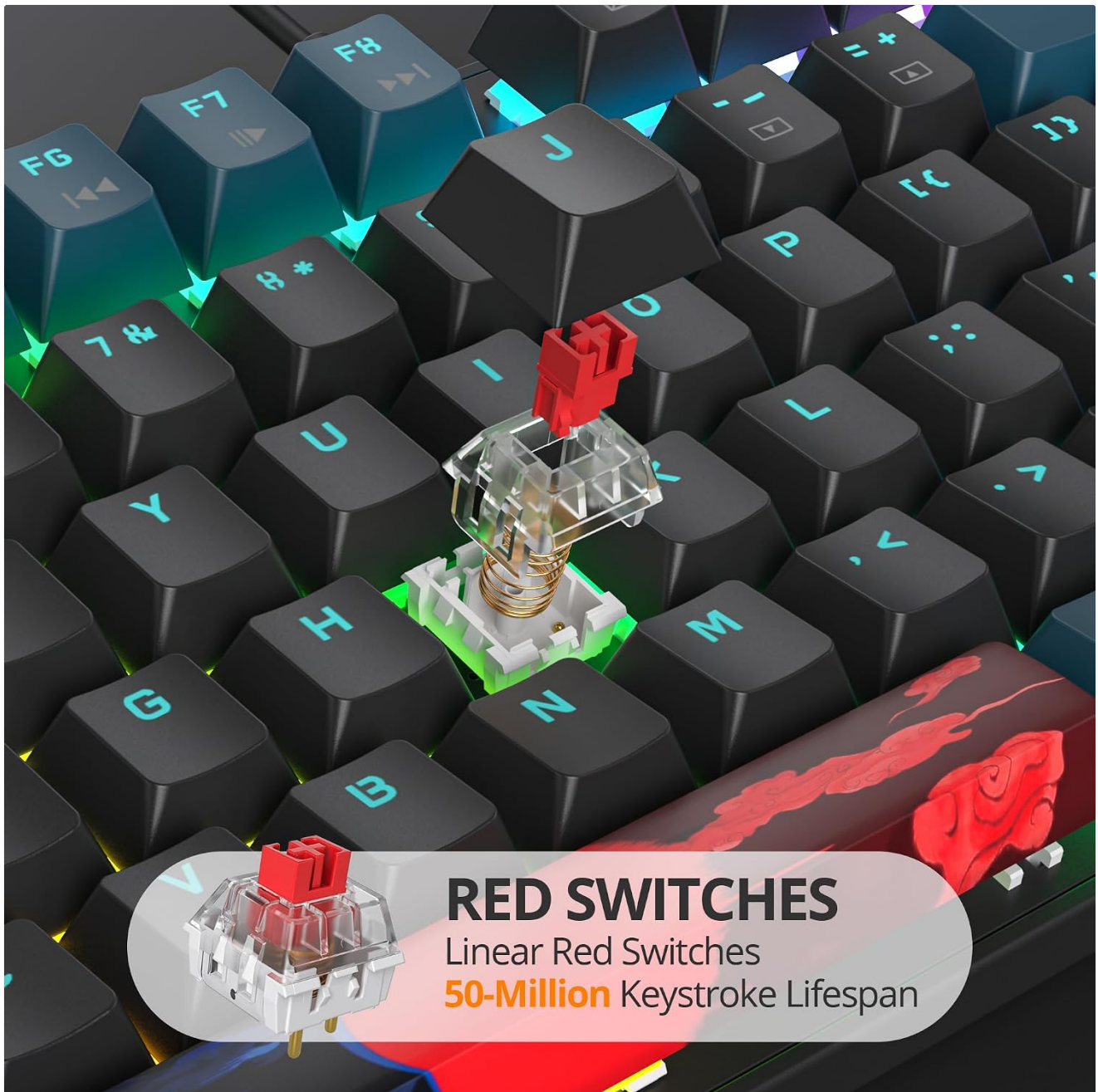
Figure 3: Close-up view of the linear red mechanical switches, highlighting their design and transparent housing.
