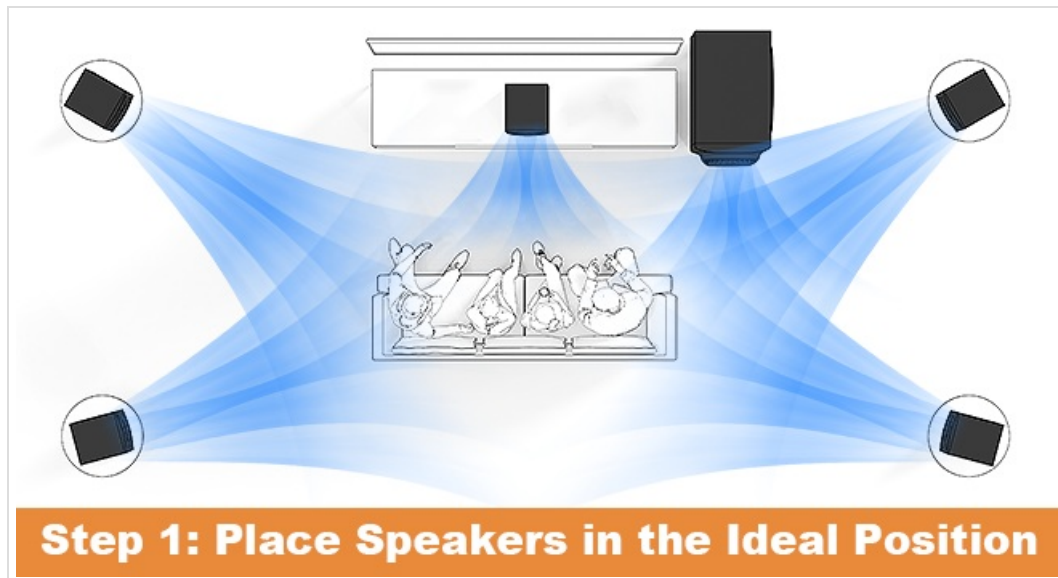
Image: Diagram illustrating the ideal placement of the subwoofer and five satellite speakers for a 5.1 surround sound setup.
