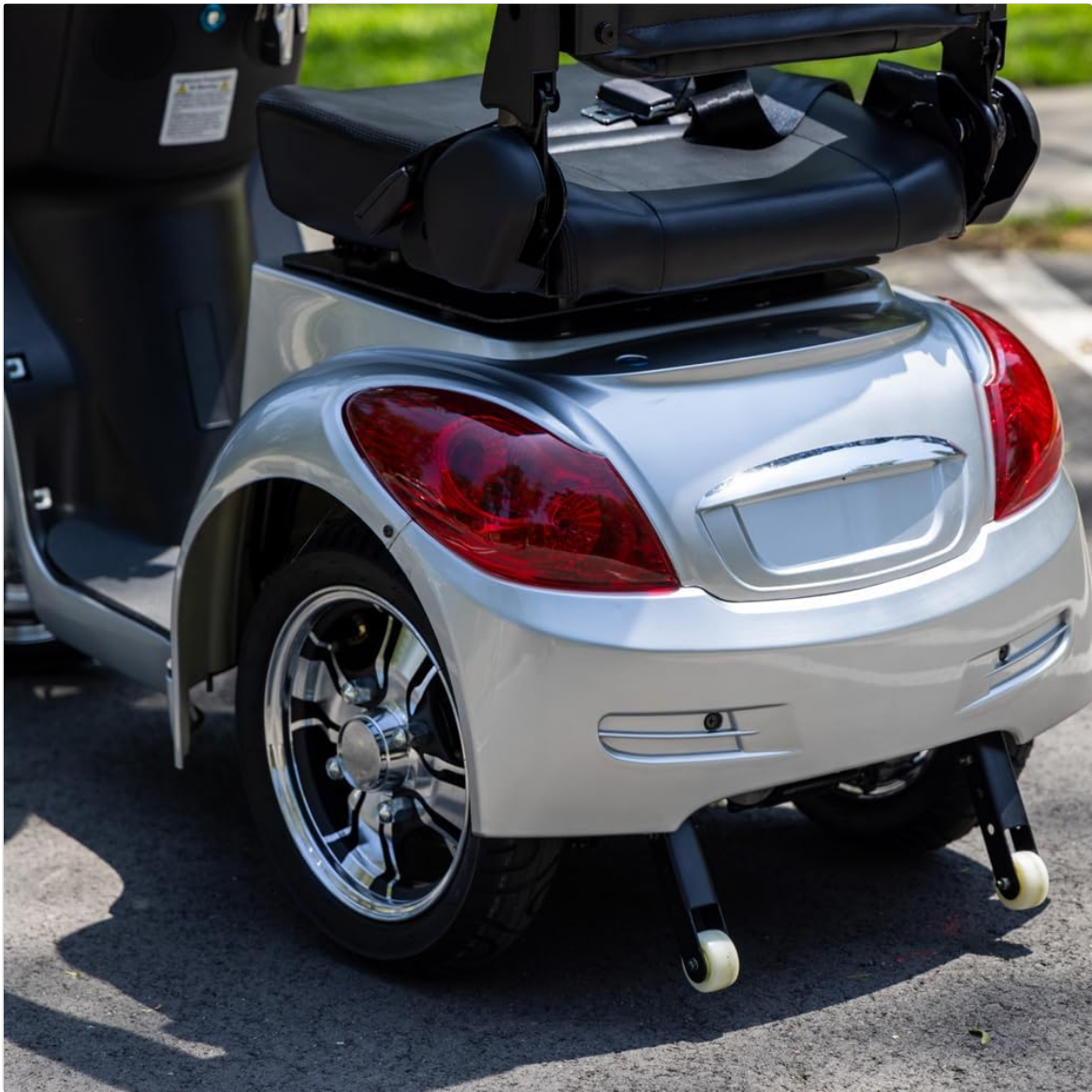
Figure 2: Rear view of the scooter, highlighting the adjustable seat and anti-tipper wheels for stability.
