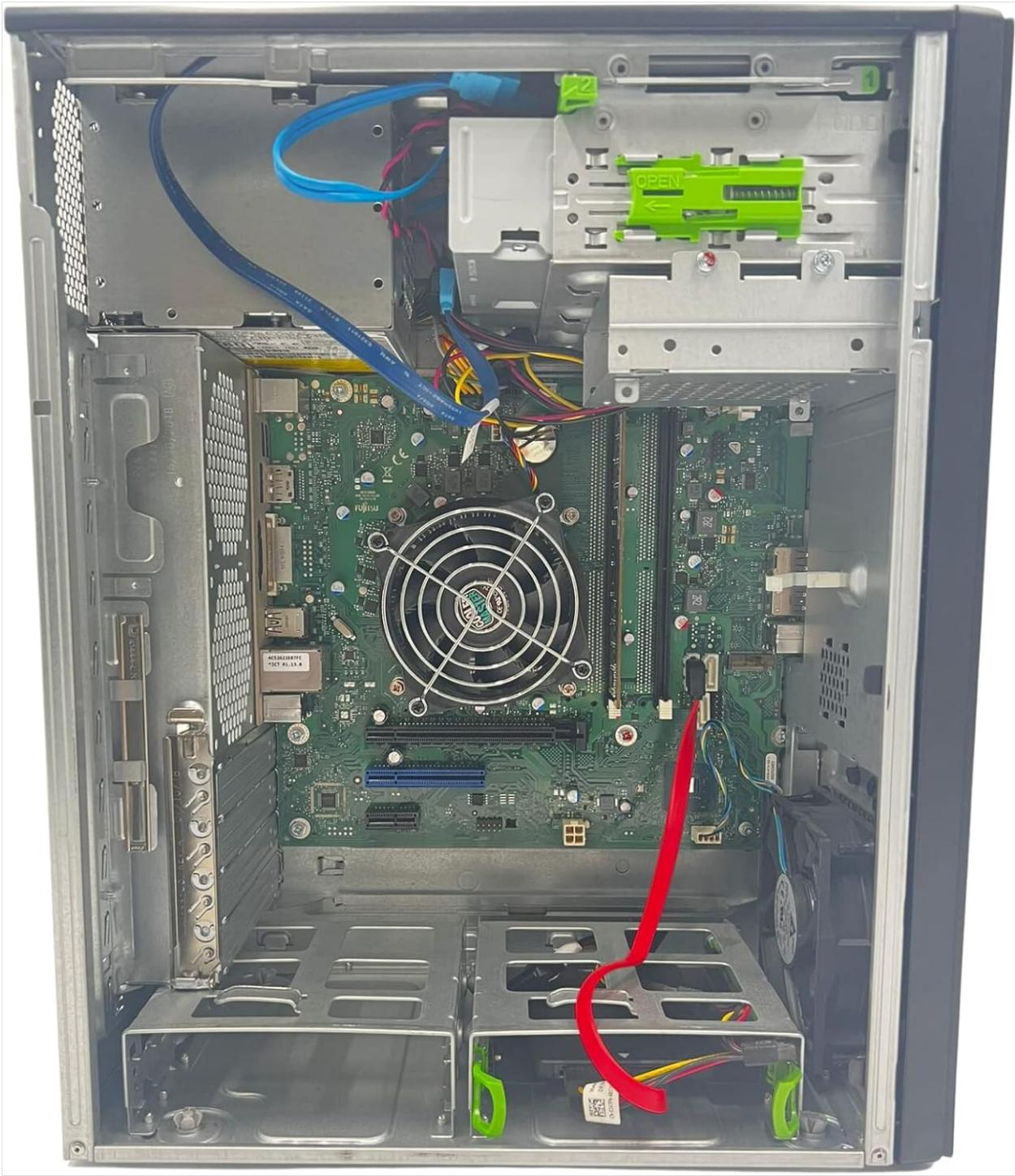
This image provides a view of the internal components of the PC, including the motherboard layout, CPU fan, RAM slots, and drive mounting areas.
